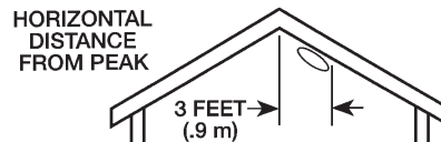
Figure 7: RECOMMENDED CO ALARM LOCATION IN ROOMS WITH SLOPED, GABLED, OR PEAKED CEILINGS.
